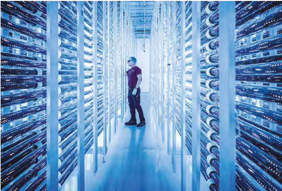
An operator runs a routine check of a photobioreactor at a microalgae facility in Reykjanesbær, Iceland, on 13 July 2020. The company uses algae to produce a food supplement rich in antioxidants. SIMONE TRAMONTE
